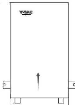
※ If you need to open the face cover, first unscrew the two screws on the side, then push it from the bottom up, and then lift it vertically up.
