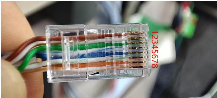
As shown in the figure: no buckle face up, from the top down, the line sequence is 12345678
