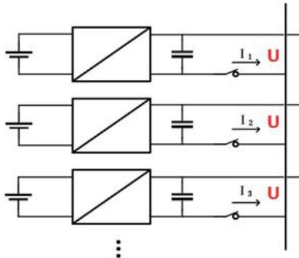
The battery packs support parallel connection, and synchronously increases the backup time or backup power.
