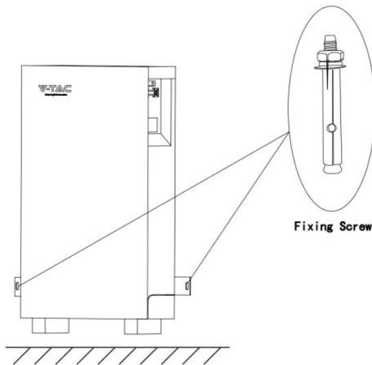
Fig.6-3 Fix the Battery to the Wall
