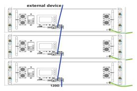
Figure 6-6 Connect 120Ω Resistor
