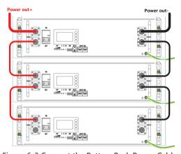
Figure 6-3 Connect the Battery Pack Power Cable
