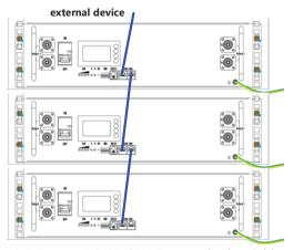
Figure 6-5 Connect RS485/CAN Communication Cable
