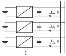
The battery packs support parallel connection, and synchronously increases the backup time or backup power.
